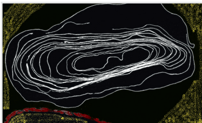
5 False coloured tomographic 'slice' through the roll prior to unrolling. White is parchment; red is linen thread; yellow is Plastazote® LD 451 foam.
